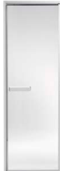
Steam Door 50 G (Art. 9091 1010) Compact model in tempered clear glass with concealed hinges. Frame size: 1855 x 635 x 43 mm. Width of opening 550 mm.
